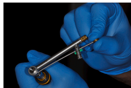
Figure 3. Marker being used when verifying torque device appropriately calibrated. Verification device held in one hand.
